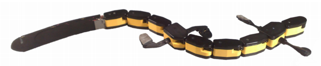
Figure 1: Salamandra robotica II modular robot (Crespi 2011)
