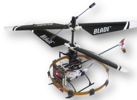
Autonomous MAV with custom sensor ring
