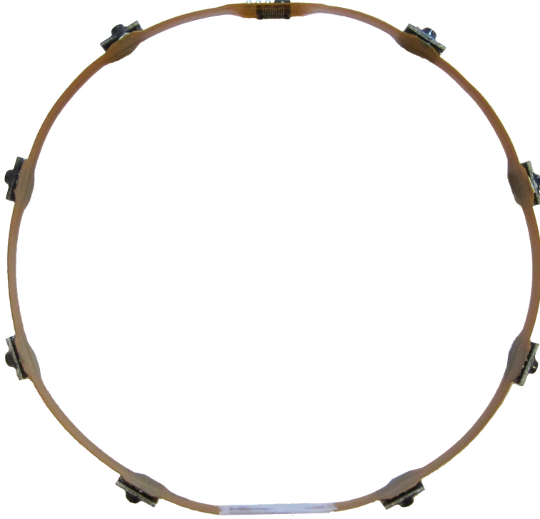
Figure 9: Optic flow sensor ring (actual size)
